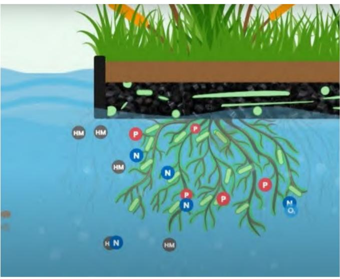
Graphical Representaiton of how floating wetlands create a filteration system that absorb harmful nutrients and heavy metals from the waterbodies, and how biomedia and roots provide surface area for growth of beneficial bacterial cultures
